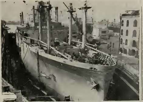
The Panama Liner Cristobal in dry dock at Todd Shipyards Corporation's Brooklyn Division undergoing final stages of reconversion.
